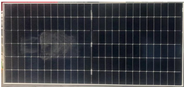
Sample 3#: Burning brand test (front)
