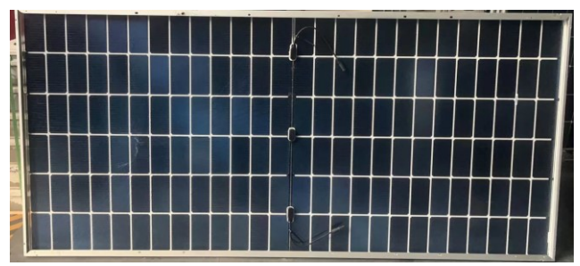
Sample 3#: Burning brand test (back)
