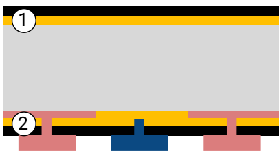
Fig.: Cross-section of a conventional cell
