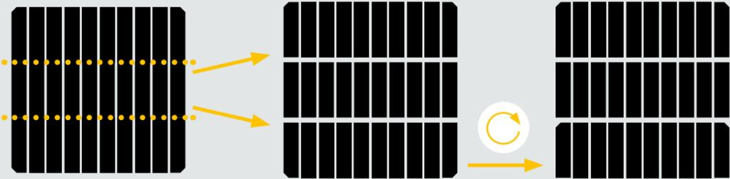
Solar modules with halved solar cells are known as half cell modules or halfcut solar modules. This generation of solar cells has advanced properties.
